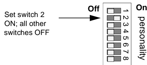
Figure 1-13. Placing Cyberlight fixture in setup mode allows you to perform the necessary lamp optimization prior to using a newly-installed lamp.
